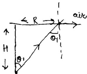
For light not to escape the water, the max angle of incidence can lead to critical angle.
