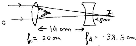
An object placed at infinity will form its image in the focal pt. of the convex lens.
